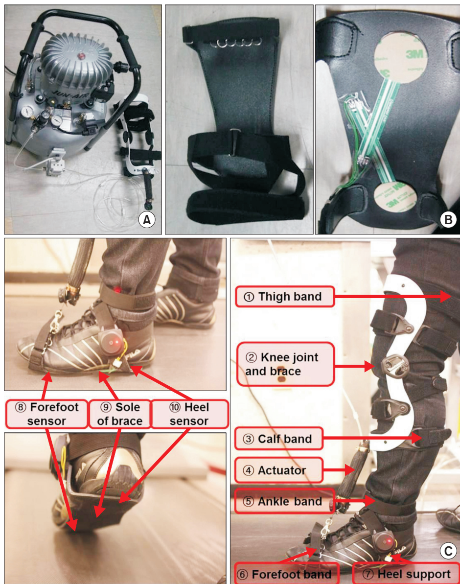
Fig. 1. Components of powered knee-ankle-foot orthosis. The actuator (A) was activated by pushing sensor on forefoot and heel (B) of a powered knee-ankle-foot orthosis (C).
