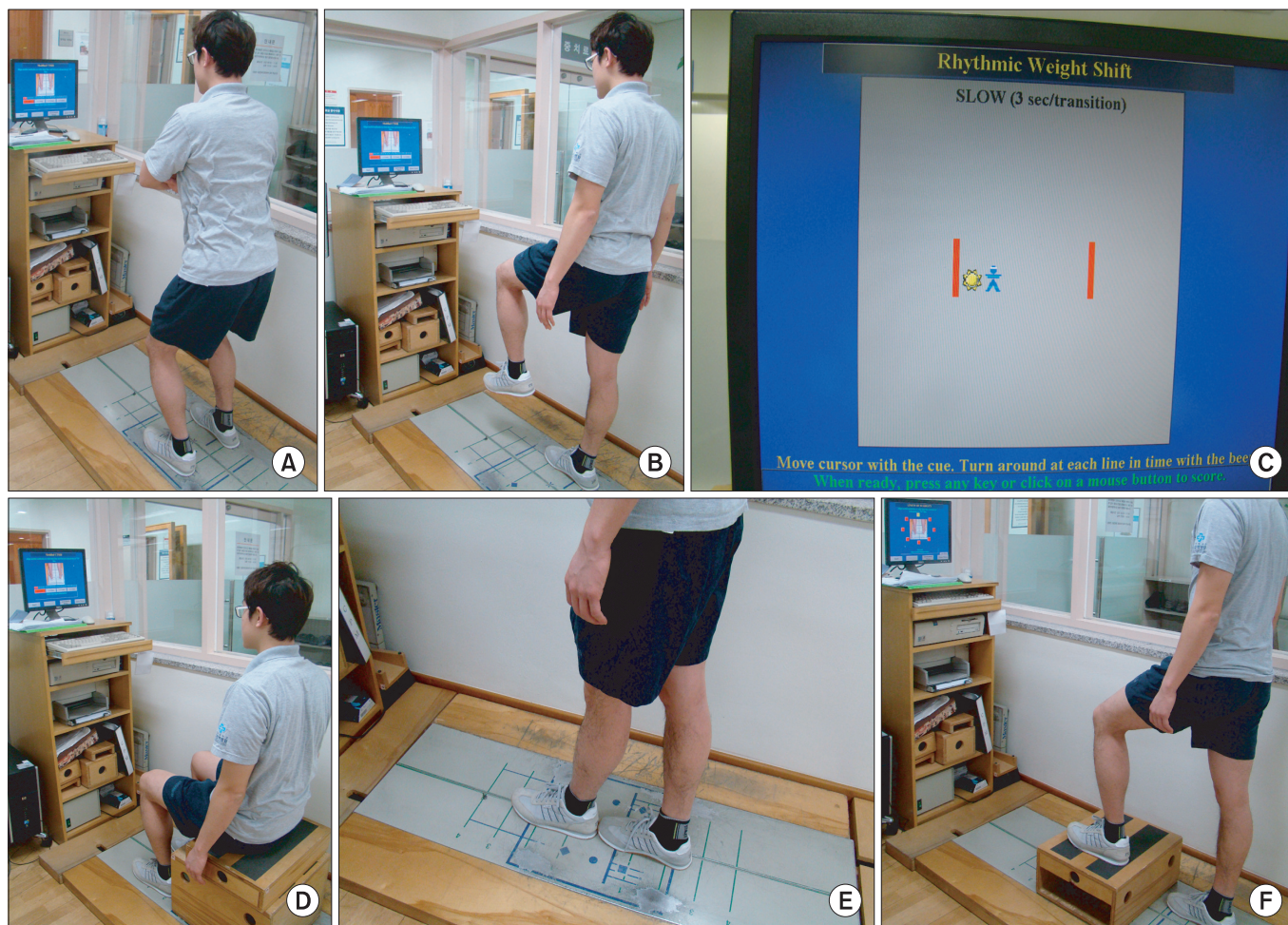
Fig. 1. Computerized posturographic measurement using the Balance Mater System®, which consists of a force platform and a computer. Using this system, we measured the weight bearing pattern (A), sway velocity of center of gravity (COG) of the body during one leg standing (B), on-axis velocity and directional control during rhythmic weight shift (C), rising index during sit-to-stand (D), end sway during tandem gait (E), and movement time during step up/over task (F).
