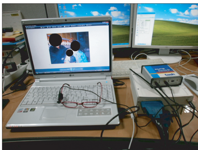
Fig. 1. A picture of the microswitch including the optic sensor connected on the eyeglasses.
